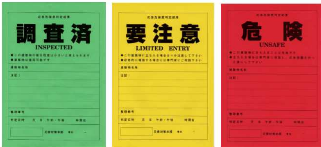
Figure 10: Affichettes post évaluation. Source: Japan Council for Quick Inspection of Earthquake Damaged Building
