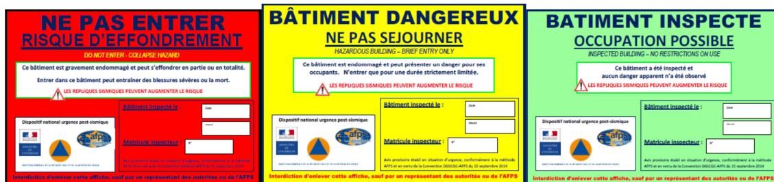
Stickers developed by AFPS to identify inspected buildings
